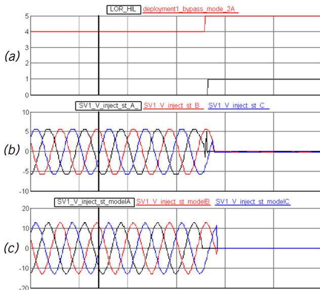
Demonstration of low overcurrent ride through feature via RSCAD simulation
