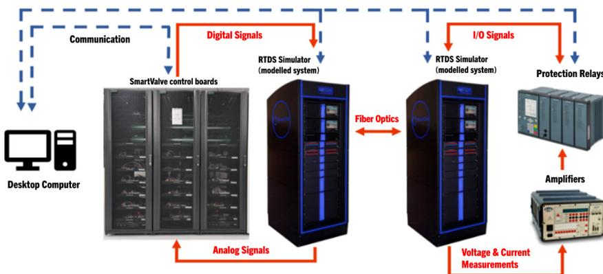
In this HIL setup, Smart Wires connected one NovaCor® chassis to the SmartValve control boards and the second chassis to protective relays. Both the SmartValve and the protection receive analogue output signals from the simulation and provide responses via digital inputs. A power amplifier is required to amplify the  $\pm 10 V_{peak}$  analogue signals from the RTDS Simulator to secondary-level signals for the relays.
