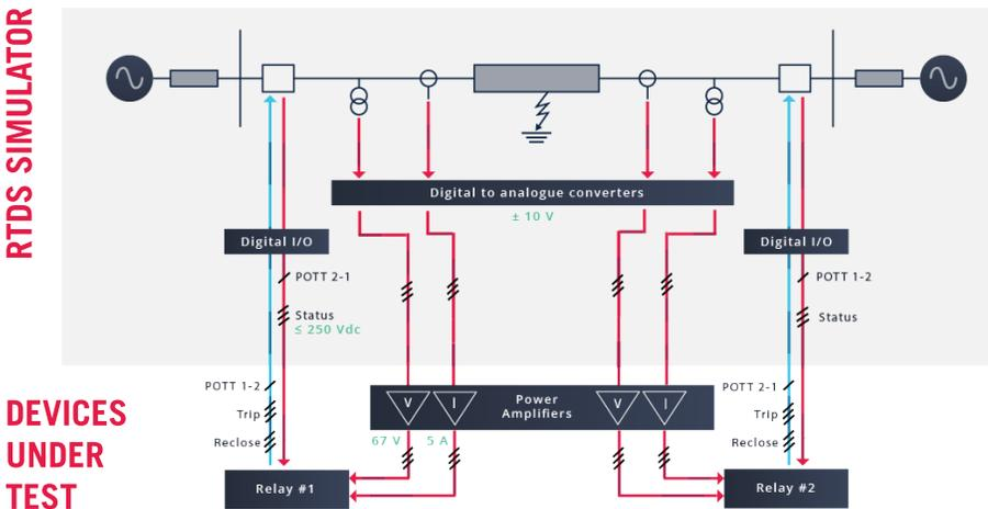
Typically, detailed models of the instrument transformers (CT, PT and CVTs) are used to provide signals to digital to analogue (D/A) converters.
