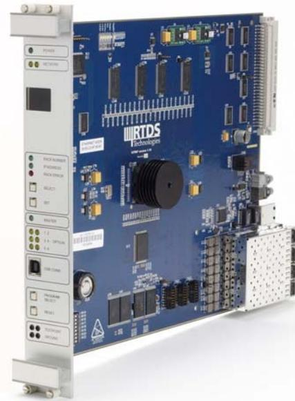
Each GTWIF has six optical fiber ports for IRC communication (the same number as the existing IRC card) to allow full interconnection of 7 rack simulators. Development is also nearly complete on the IRC Switch which will allow direct communication between as many as 60 simulator racks.
