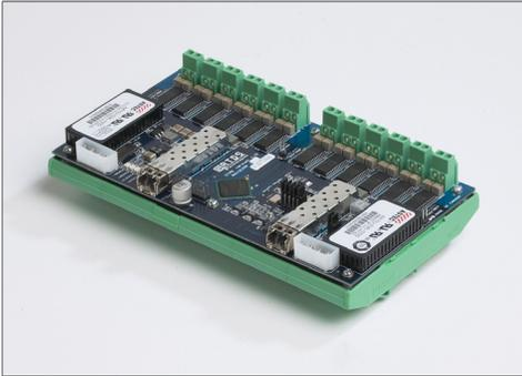
The GTAO provides optically isolated analogue output from the simulation to external equipment. The card has a total of 12 outputs which can be sent from either regular or small timestep simulations running on the PB5.
