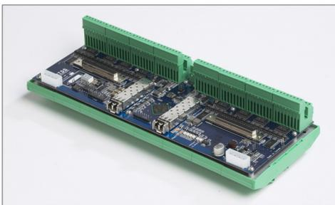
The GTDO provides optically isolated digital output from the simulation to external equipment. The card has a total of 64 outputs which can be sent from either a regular or small timestep simulation running on the PB5 card.
