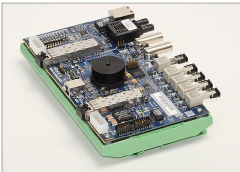
The GTSYNC card is used to synchronize the RTDS simulation timestep to an external time reference (eg. GPS clock) and to synchronize devices under test. The GSYNC connects to the GT port on the GTWIF and cannot be daisy chained to other I/O cards.
