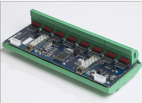
The GTDI provides optically isolated digital input to the real time simulation from external equipment. The card has a total of 64 inputs for use in regular or small timestep (1-2  $\mu$ s) simulations running on the PB5 card.
