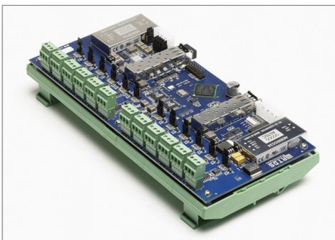
The GTAI provides optically isolated analogue input from external equipment to the simulation. The card has a total of 12 true differential inputs which can be read by simulation components running on the PB5.
