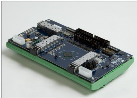
The GTFPI card is used to read and write signals between the front panel and the RTDS Simulator. The GTFPI can be used with both the TTL level digital I/O panel and the dry contact (high voltage) panel.
